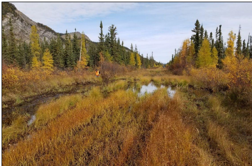
Photo 7: Drainage #5 looking north Approximately 4 L/s flowing to the east. Pooling of water extends downstream (east) of the alignment as no defined channel exists
