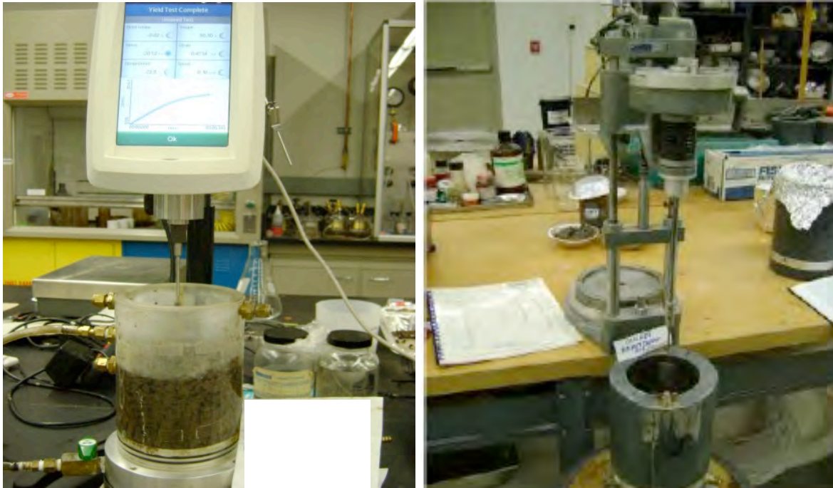
Figure 3. A; Rheometer and B: Vane shear apparatus
