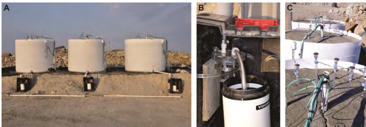
Figure 2 Photos showing (A) completed PK tanks, from left to right FT, MT, CT (B) tank bottom drain pipe discharging into the sample cell and tipping bucket (C) instrumentation on tank tops.
