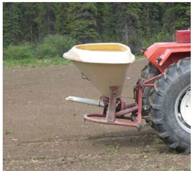
FIG 4.14 Fertilizer and seed are usually applied to the ground surface using a broadcast spreader, after which they are worked into the soil with a harrow. The broadcaster on top is a cyclone type spreader and the one on the bottom is a pendulum spreader.
