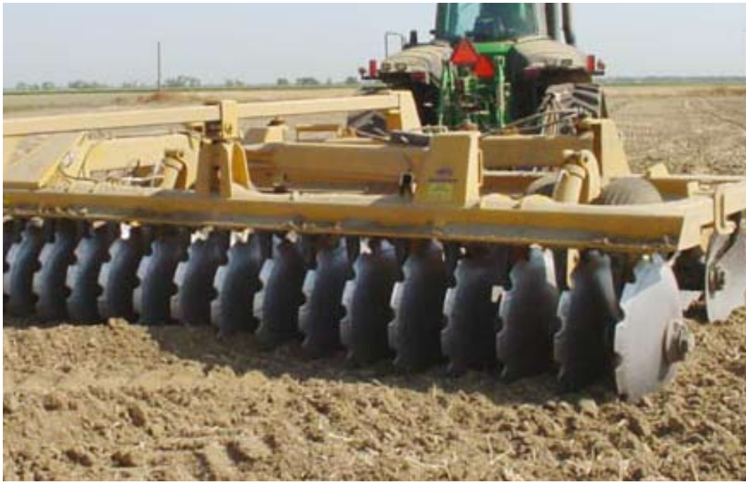
FIG 4.16 Large sites will call for large equipment, such as this tandem disk harrow, to prepare soil.
