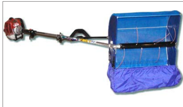
FIG 4.27 Specialized equipment, such as this harvester fabricated from a weed-trimmer, is available for collecting wild seed.
