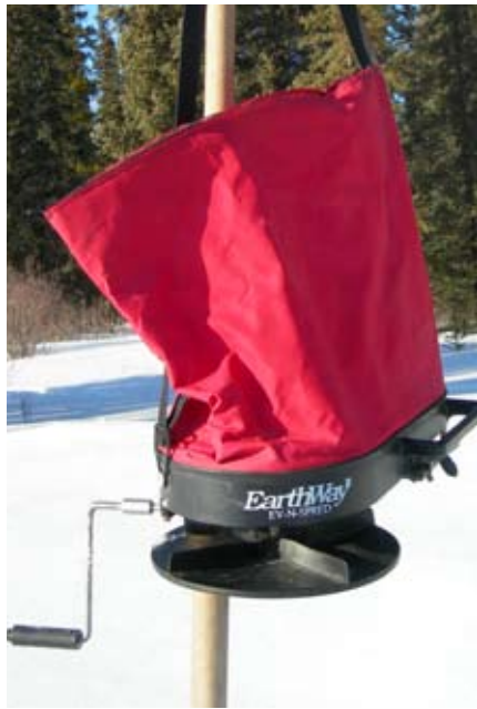
FIG 4.22 Hand-held seeders are useful on small and remote sites. They also are valuable for spot seeding on any type of site.
