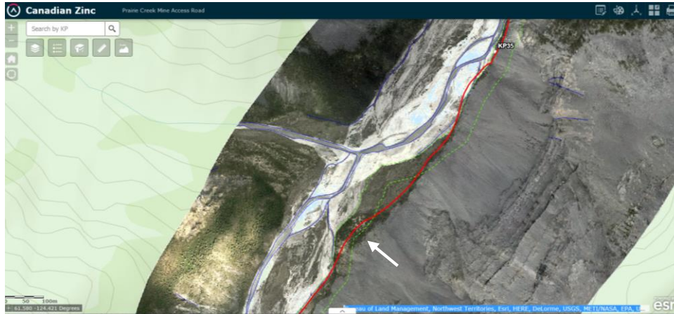
Figure 9 Sundog Creek at Km 34.7 – ortho photo showing road (red) and 50 m riparian area (green).
