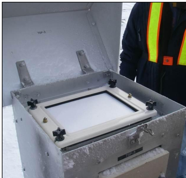
Plate 5.1-2. HVAS station TSP-3, exposed filter view, May 2011.
