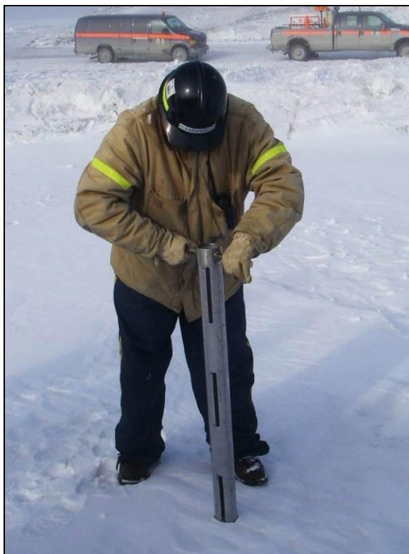
Plate 5.4-1. Snow core sample being collected with a Mt. Rose snow core sampler.
