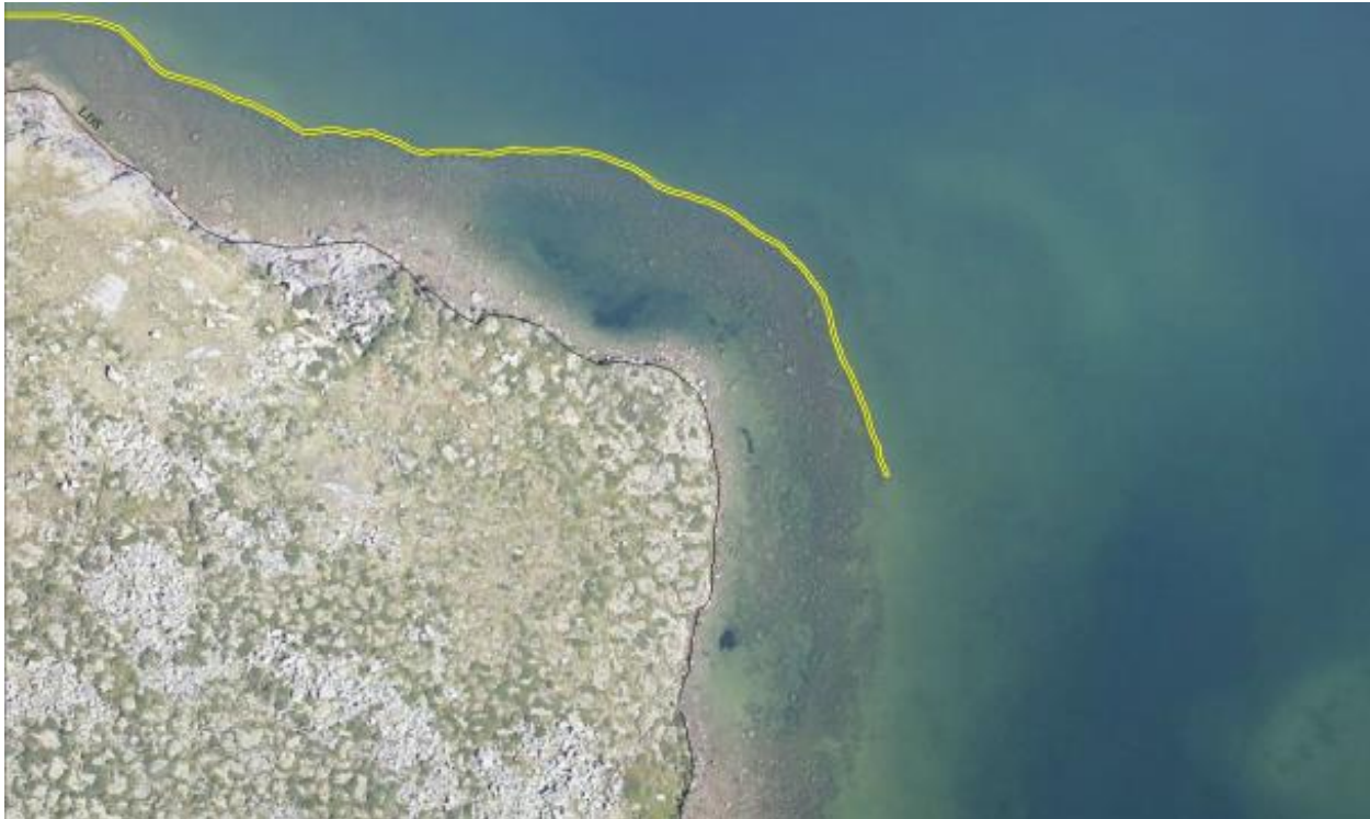
Figure 3.1-1 An Example of Digitizing Substrate Using Orthophotos
